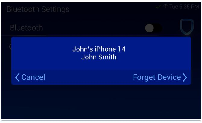
Note: Up to 6 devices can be paired to the keypad. This feature is a per keypad operation. To use Bluetooth disarming at multiple keypads on a system, you will need to individually pair the device at each keypad you want to automatically disarm.
