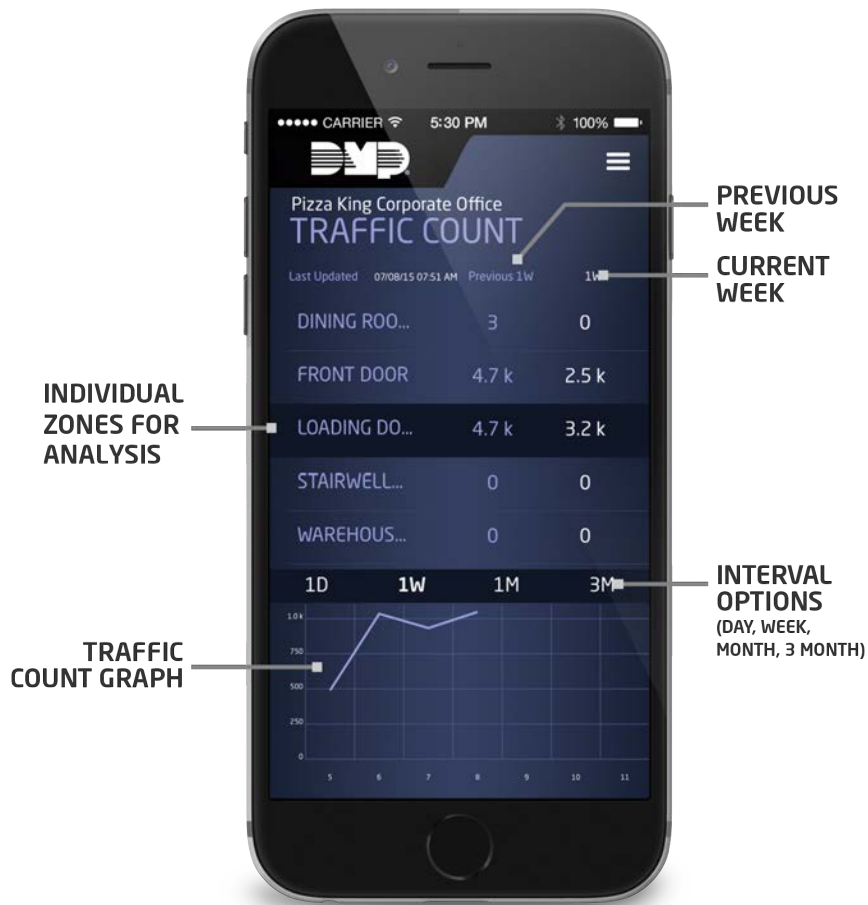
DMP Traffic Count feature screen shot showing previous-to-current week comparison for five zones
