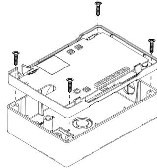
Figure 9: Mounting the TMSentry to the Backbox
